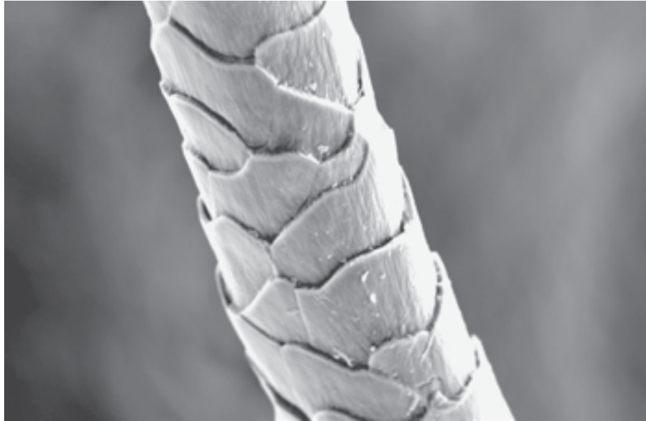
Above: Wool fibre at microscopic level showing overlapping scales
